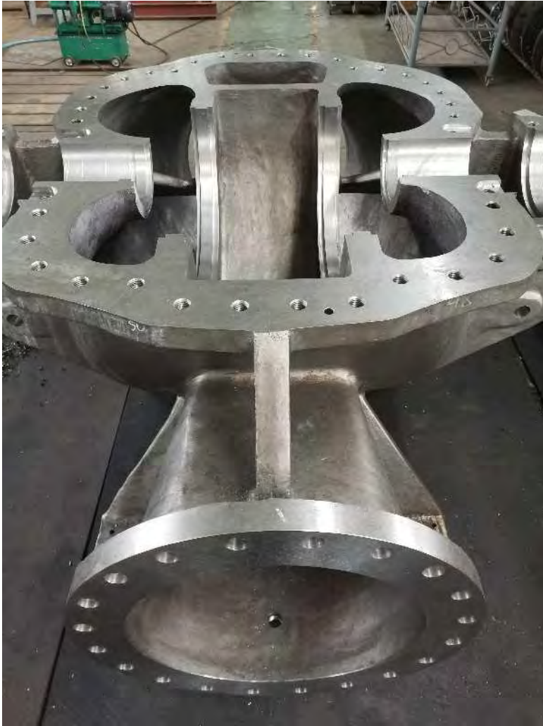
Casing. Size 24x30-32 Casing. Casting, 3 D Drawing, Manufacturing, Delivery to USA. PROJECT No. 81053J
